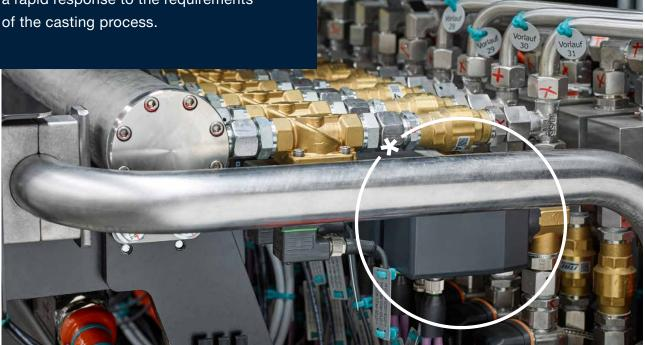
a sort of visitor's card for the part." The valve set-points, conveniently defined by software, are stored under password protection and can easily be selected by the operating staff at the machine interface. The cooling process can therefore be effortlessly adapted for Fill's customers to meet the requirements of different parts to be produced. There is no need for time-consuming resetting of the flow values, scrap is reduced.
