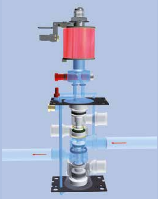
Switched position of the 5/2-way valve
