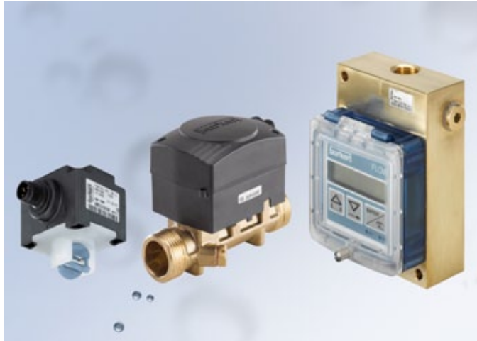
Fig. 4: Sensor technology for electrode clamp cooling (from left) Paddle wheel sensor for systems with 4-20 mA/frequency and switching output Ultrasonic sensor with 4-20 mA or frequency output Dual paddle wheel sensor for separate flow monitoring at each electrode cap
