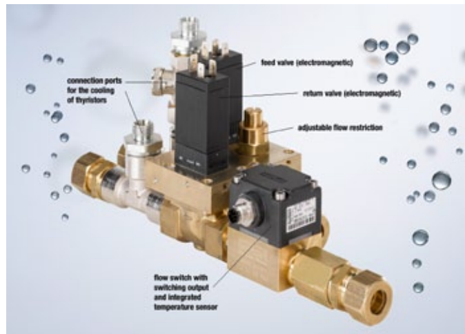
Fig. 3: Cooling water monitoring block with solenoid valves and flow sensor with integrated temperature sensor
