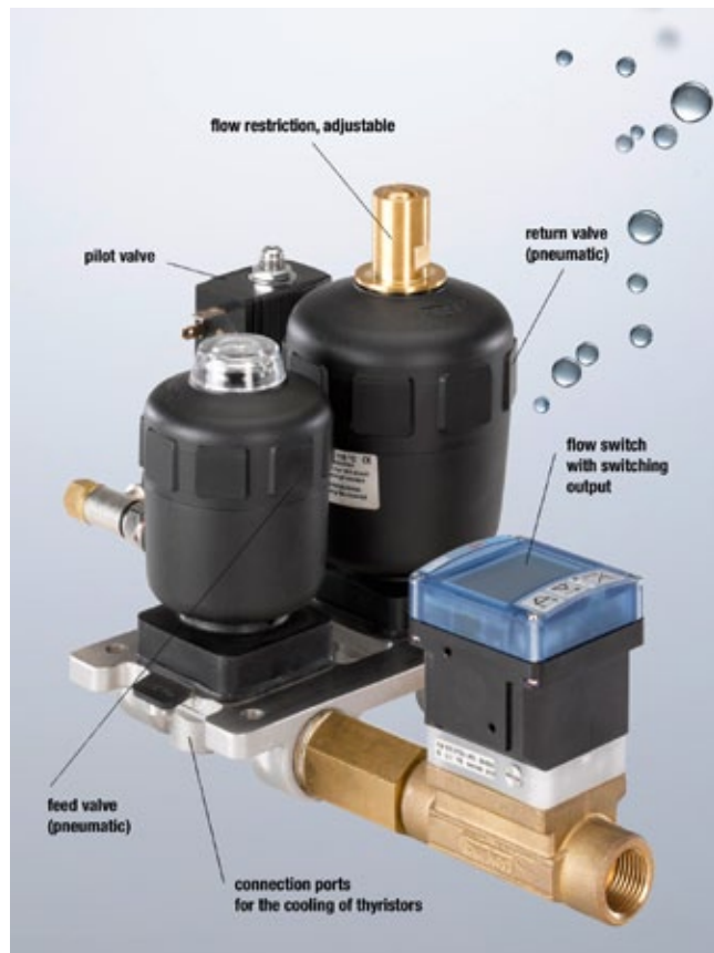
Fig. 1: Cooling water monitoring block with diaphragm valves and flow switches
