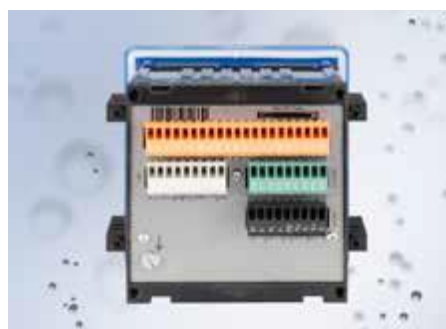
Back side of the Bürkert MultiCELL 8619 controller with SD card slot, mainboard (orange), signal input card for pH/ORP (white), signal input card for conductivity (green) and signal output card (black). The three free slots are protected by the metal plate
