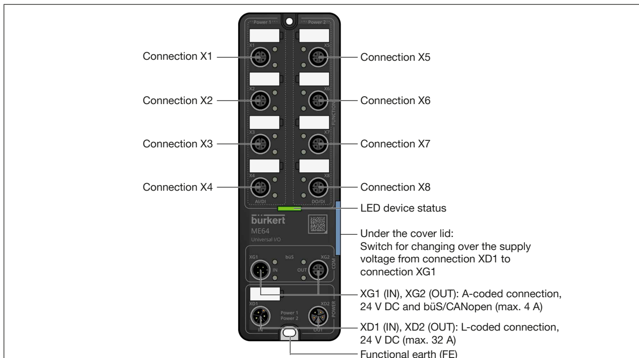
Figure 1: View of the I/O module, Type ME64 universal I/O
