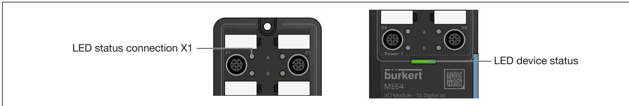
Figure 20: Type ME64 Universal I/O display elements
