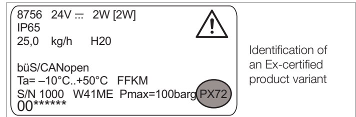
Fig. 1: Location of the variable key PX72 on the Type label
