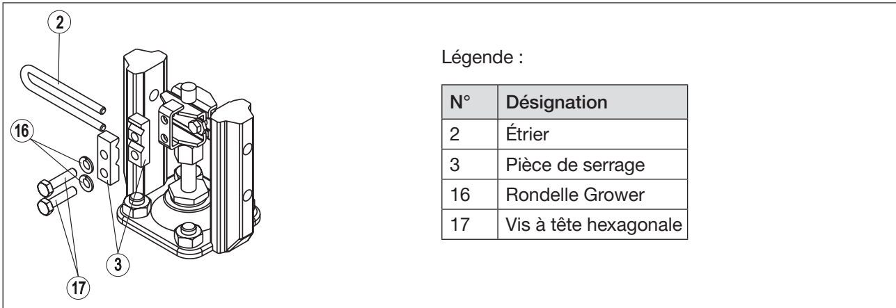
Figure 16 : Installation de l'étrier
