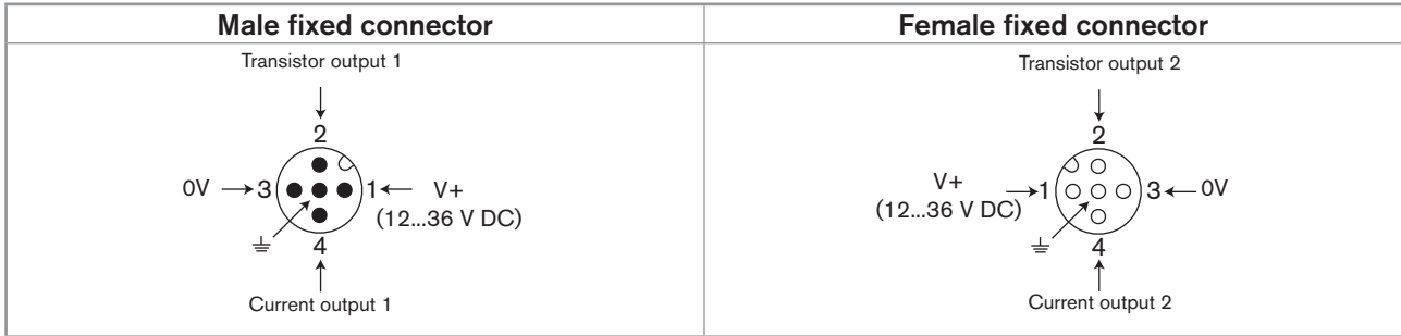
Fig. 21 : Pin assignment of the male and female M12 fixed connectors
