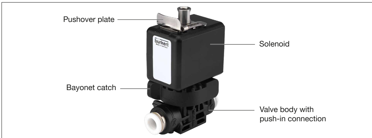
Fig. 2: Device with push-in connection
