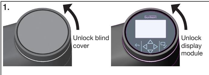
Fig. 17: Remove blind cover or display module
