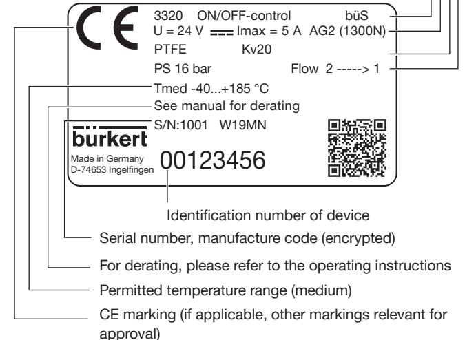
Fig. 4: Description of the type label (example)
