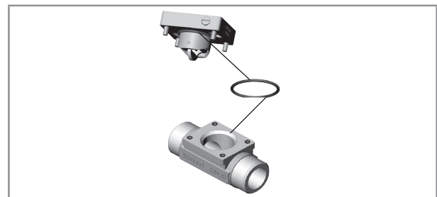
Fig. 6: Position of O-ring in an S039 fitting
