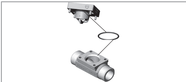
Fig. 5 : Position of O-ring in an S030 HT fitting
