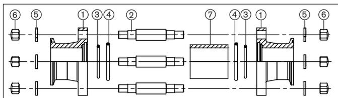
Fig. 4: Assembling full view inline inspection glass
