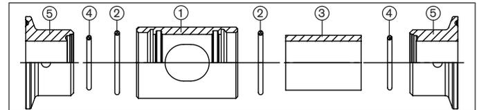
Fig. 3: Assembling standard inline inspection glass
