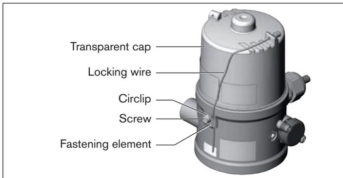
Fig. 4: Installation locking wire
