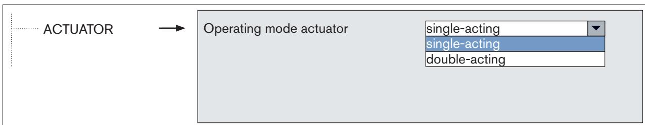
Figure 25: ACTUATOR function
