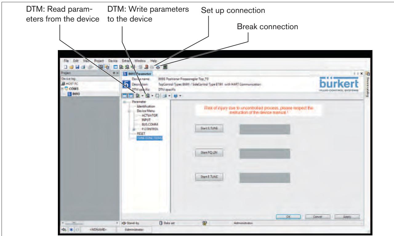
Figure 23: Transferring parameters
