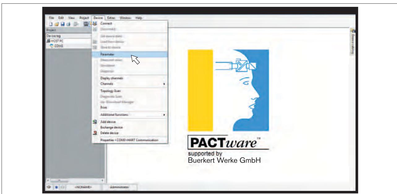
Figure 14: HART communication DTM - set parameters
