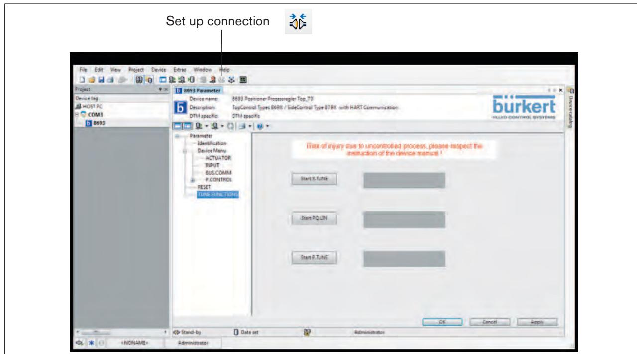
Figure 21: Starting **TUNE FUNCTIONS**
