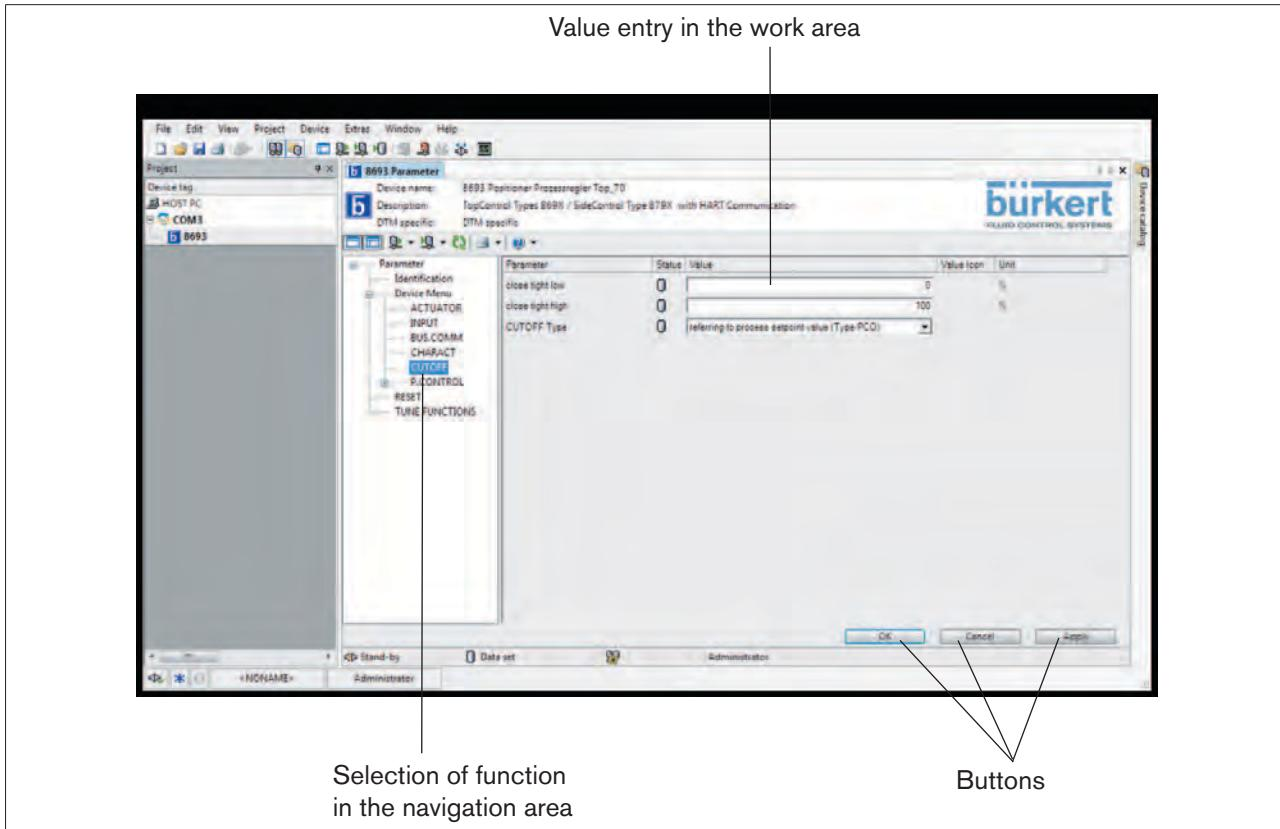
Figure 24: Parameterizing functions
