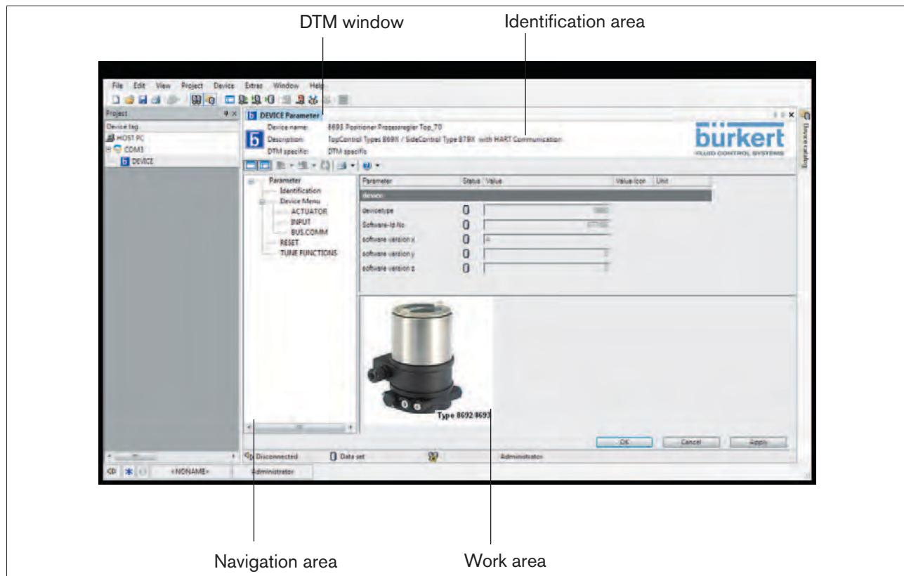
Figure 18: DTM window
