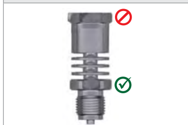
Mounting a cooling element
