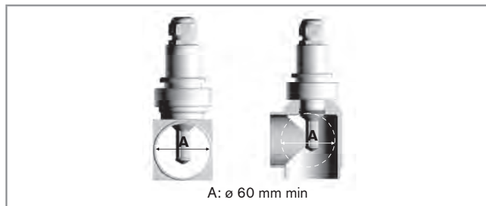
Fig. 11: Placing the product onto the pipe
