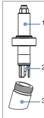
**1:** G 1 1/4" probes holder Type 8200 with O-ring position of 28 mm or 46 mm
