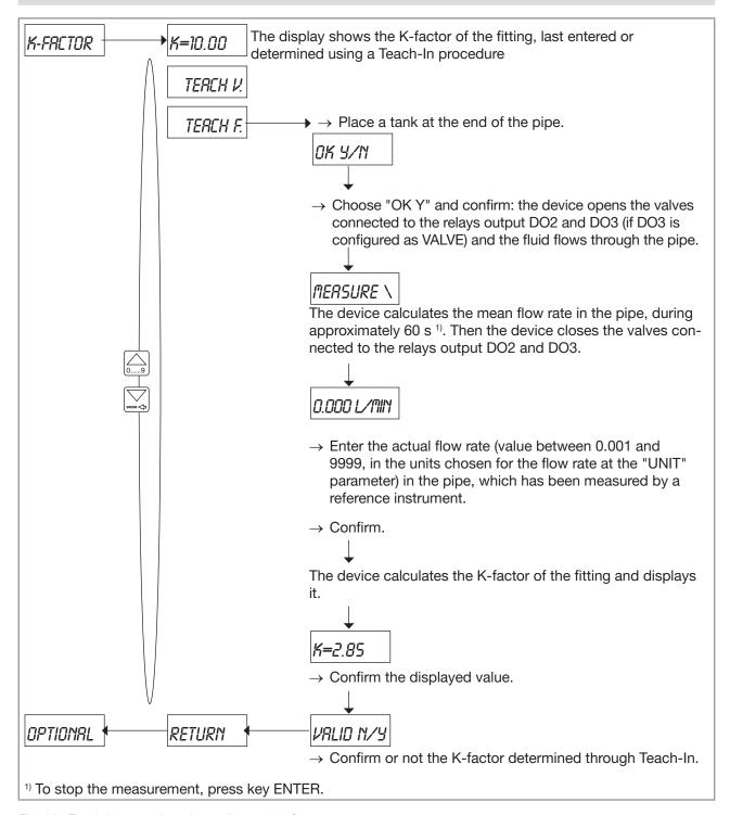
Fig. 62: Teach-In procedure depending on the flow rate
