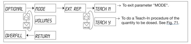
Fig. 70: Configuring the dosing mode "EXT. REP."
