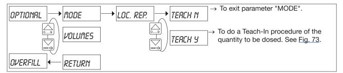
Fig. 72: Configuring the dosing mode "LOC. REP."
