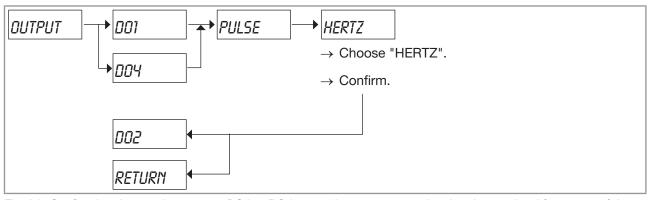
Fig. 84: Configuring the transistor output DO1 or DO4 as a pulse output propotional to the rotational frequency of the paddle wheel
