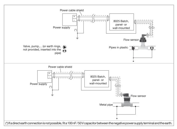
Fig. 21: 8025 Batch in panel-mounted or in wall-mounted version, equipotentiality skeleton diagram
