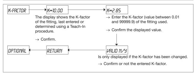
Fig. 60: Entering the K-factor of the fitting used
