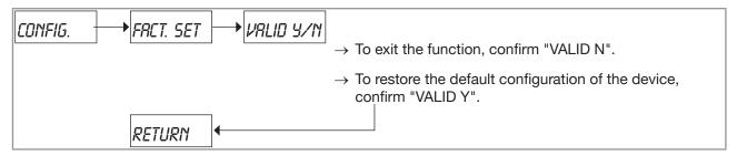
Fig. 102: Restoring the default configuration of the device
