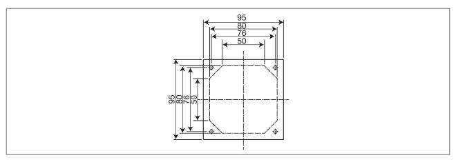
Fig. 16: Dimensions [mm] of the electrical cabinet frontage cutting plan
