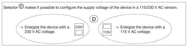
Fig. 30: Selector of the supply voltage on a 115/230 V AC version
