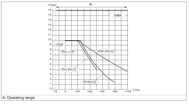
Fig. 9: Fluid temperature/fluid pressure dependency curves for a dosing controller type 8035 Batch, depending on the material the S030 sensor-fitting is made of
