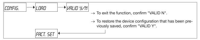
Fig. 101: Restoring the configuration previously saved
