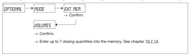
Fig. 67: Configuring the dosing mode "EXT. MEM."
