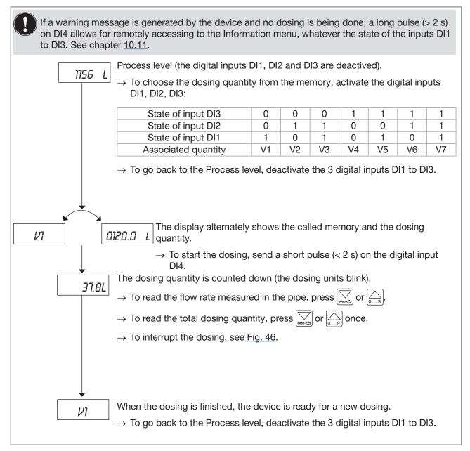
Fig. 48: Doing a dosing of a quantity from the memory via the digital inputs, in dosing mode "EXT.+LOC."
