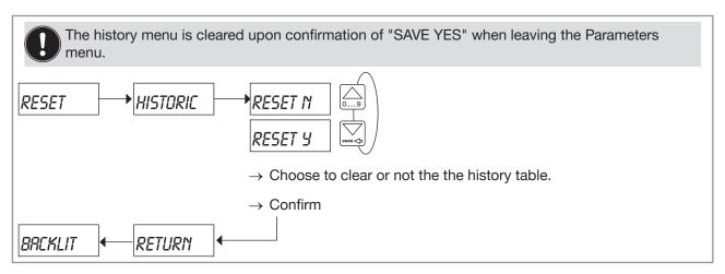
Fig. 91: Diagram of the "HISTORIC" parameter of the sub-menu "RESET"
