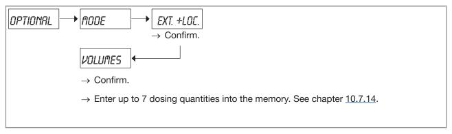
Fig. 68: Configuring the dosing mode "EXT. +LOC."
