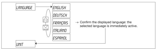
Fig. 58: Diagram of the "LANGUAGE" parameter of the Parameters menu
