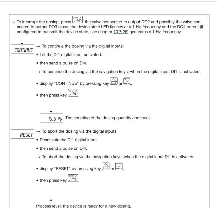
Fig. 54: Interrupting the dosing, in dosing mode "EXT. REP."
