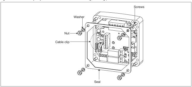
Fig. 17: Installation of the 8025 Batch in panel version
