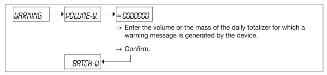
Fig. 98: Diagram of the "VOLUME-W." parameter of the sub-menu "WARNING"
