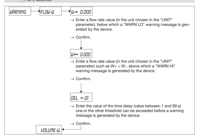
Fig. 97: Diagram of the "FLOW-W." parameter of the sub-menu "WARNING"
