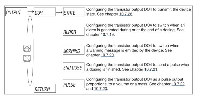
Fig. 79: Diagram 2/2 of the "OUTPUT" parameter of the Parameters menu
