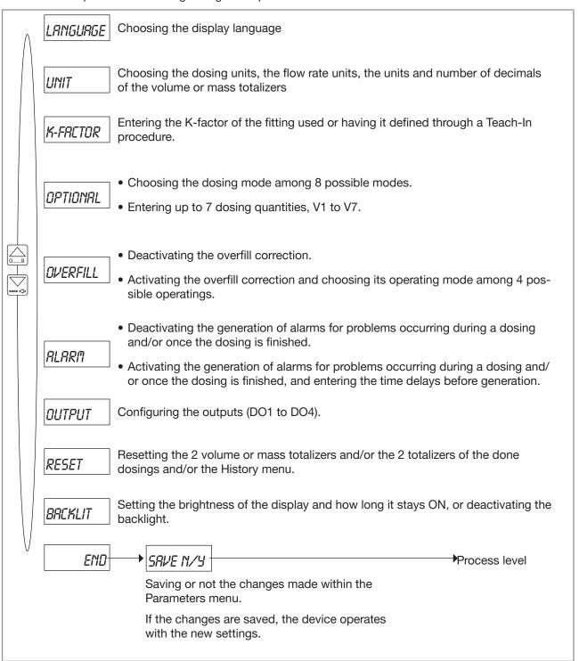
Fig. 57: Diagram of the Parameters menu
