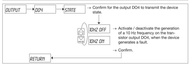
Fig. 87: Configuring the transistor output DO4 to transmit the device state
