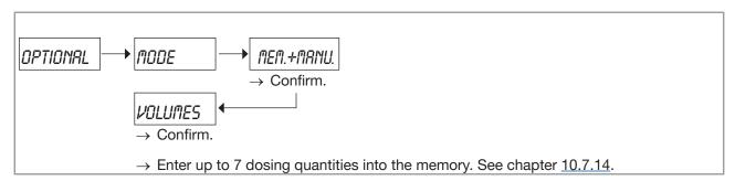
Fig. 66: Configuring the dosing mode "MEM+MANU"
