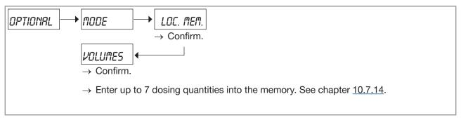
Fig. 65: Configuring the dosing mode "LOC. MEM."
