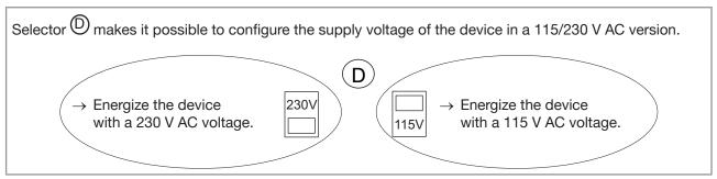
Fig. 27: Selector of the supply voltage on a 115/230 V AC version
