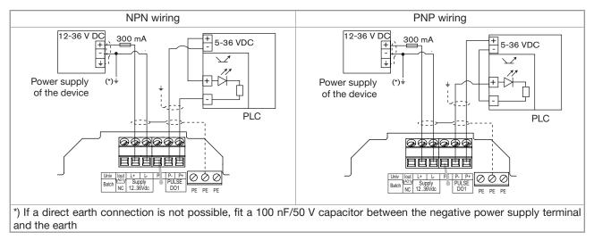
Fig. 35: NPN or PNP wiring of the DO1 transistor output of the device
