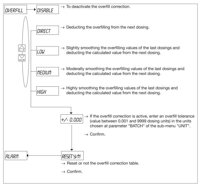
Fig. 75: Configuring the overfill correction
