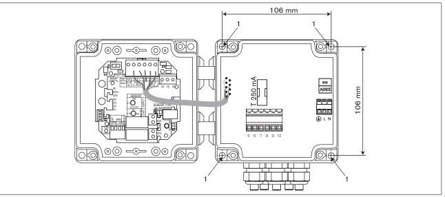
Fig. 19: Installation of the dosing controller 8025 Batch in wall-mounted version
