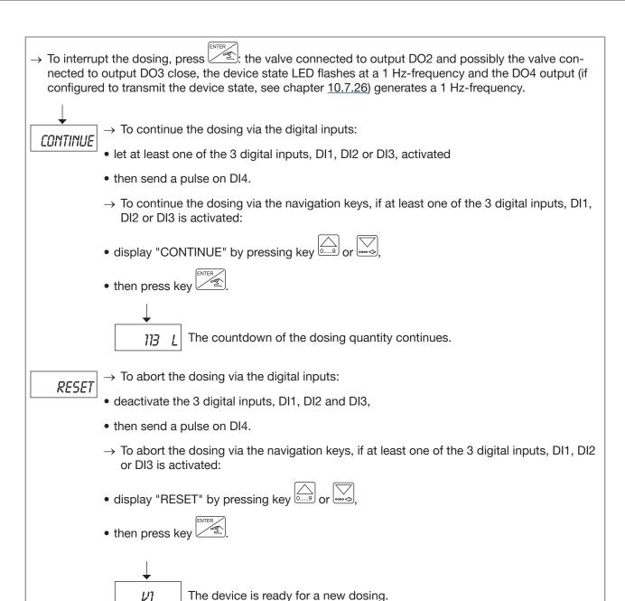
Fig. 46: Interrupting the dosing, in dosing mode "EXT. MEM."
