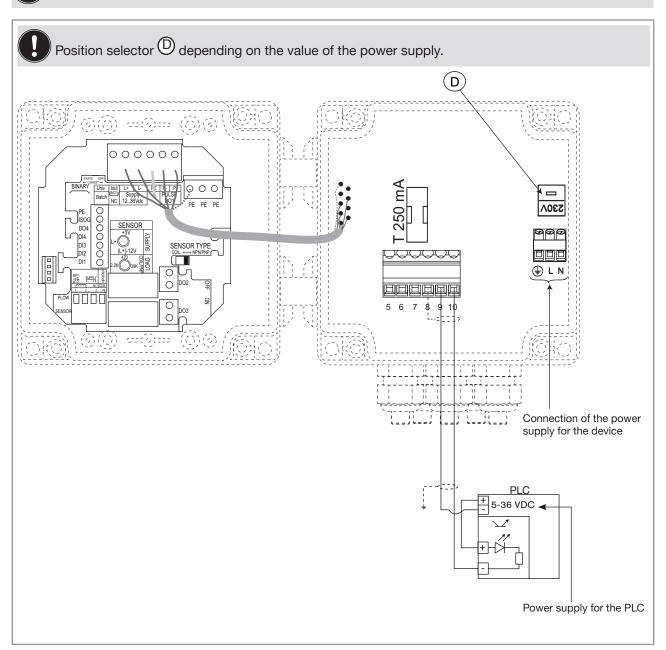
Fig. 36: NPN wiring of the DO1 transistor output of a 8025 Batch in wall-mounted version, fed with 115/230 V AC
