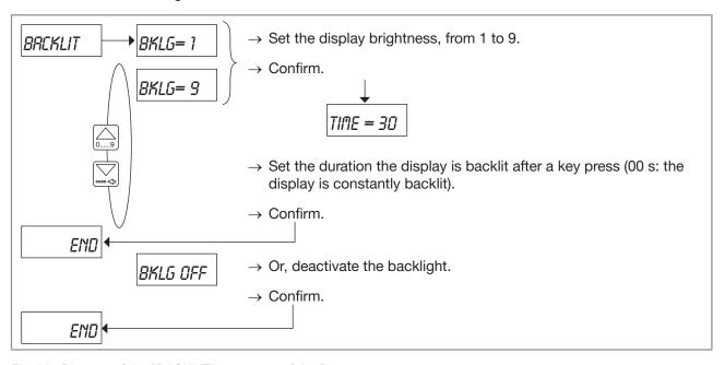
Fig. 92: Diagram of the "BACKLIT" parameter of the Parameters menu
