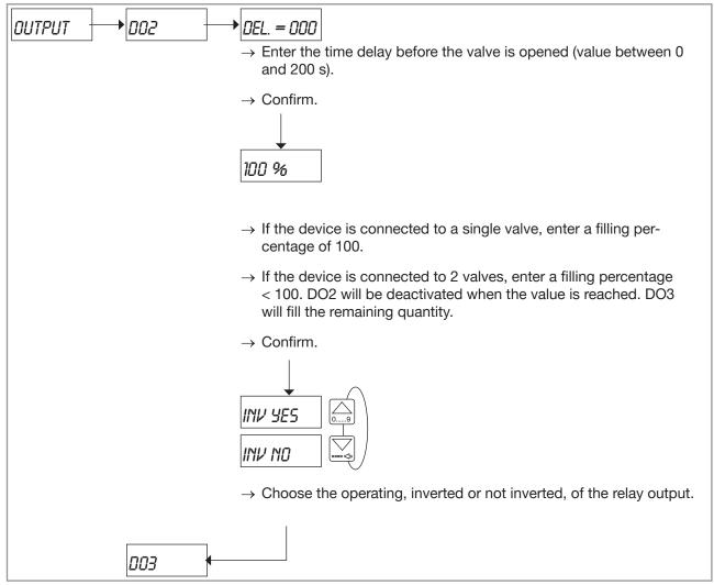
Fig. 85: Configuring the DO2 relay output
