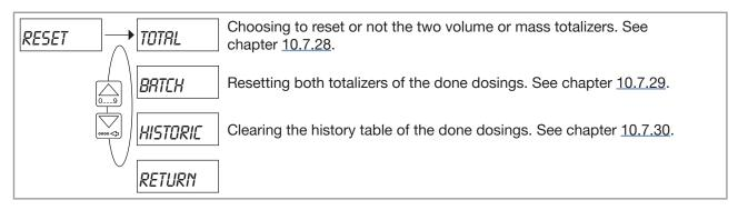
Fig. 88: General diagram of the "RESET" sub-menu
