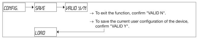
Fig. 100: Saving the current user configuration
