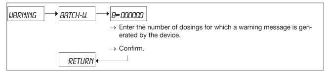
Fig. 99: Diagram of the "BATCH-W." parameter of the sub-menu "WARNING"
