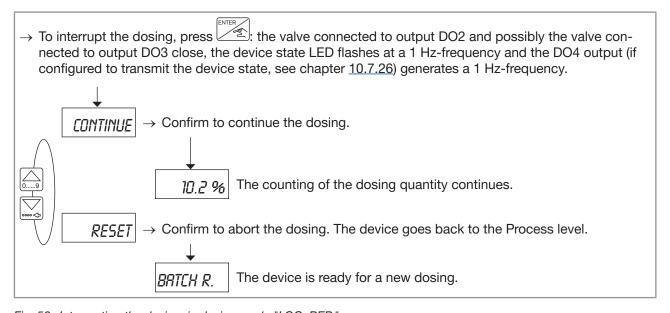
Fig. 56: Interrupting the dosing, in dosing mode "LOC. REP."
