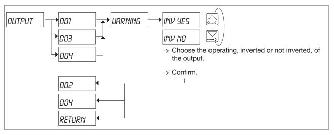
Fig. 81: Configuring the output DO1 or DO3 or DO4 to indicate the generation of a warning message
