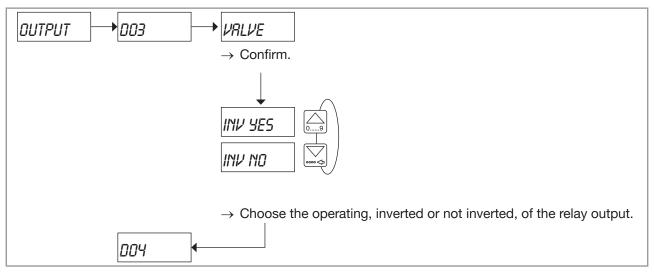
Fig. 86: Configuring the relay output DO3 to control an auxiliary valve
