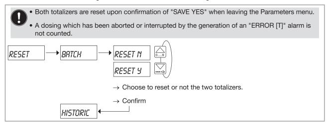
Fig. 90: Diagram of the "BATCH" parameter of the sub-menu "RESET"
