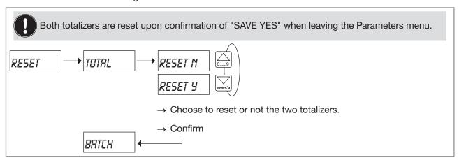
Fig. 89: Diagram of the "TOTAL" parameter of the sub-menu "RESET"
