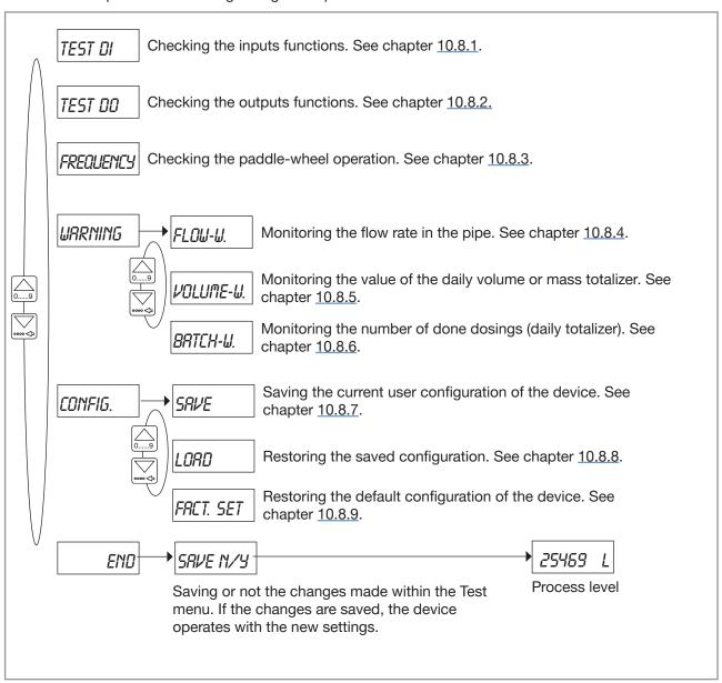
Fig. 93: Diagram of the Test menu
