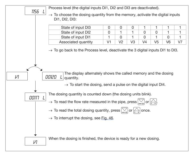
Fig. 45: Doing a dosing of a quantity from the memory, in dosing mode "EXT. MEM."
