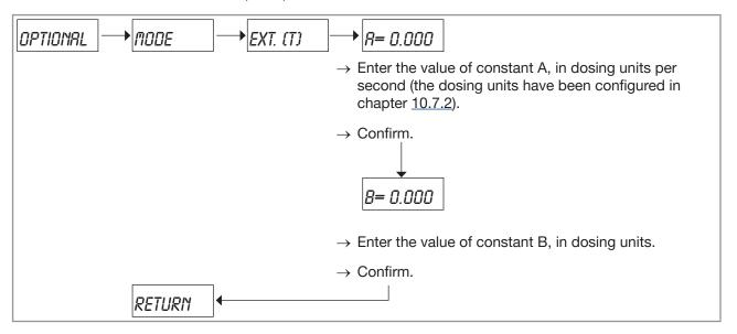
Fig. 69: Configuring the dosing mode "EXT. [T]"
