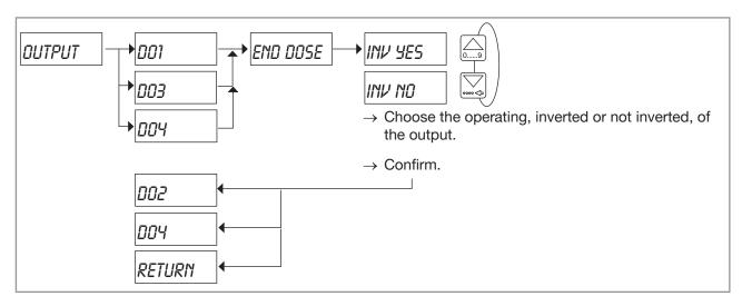
Fig. 82: Configuring the output DO1 or DO3 or DO4 to signal the end of the dosing
