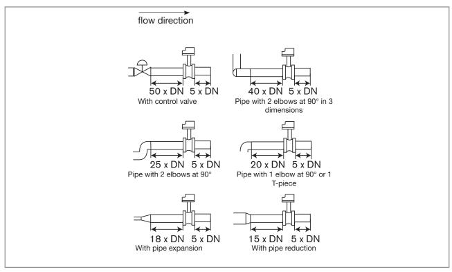
Fig. 10: Upstream and downstream distances depending on the design of the pipes.
