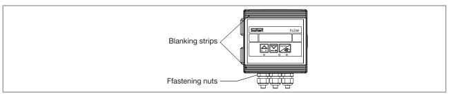
Fig. 18: Location of the fastening nuts and the blanking strips
