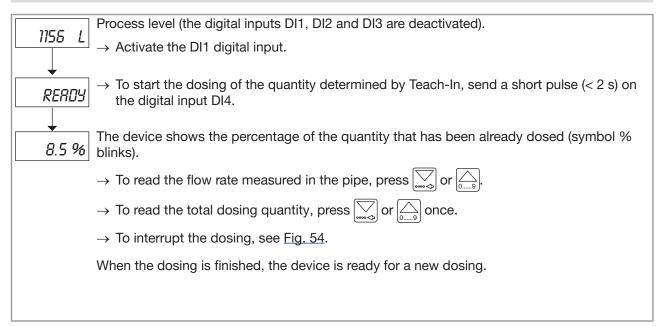
Fig. 53: Doing a dosing, in dosing mode "EXT. REP."
