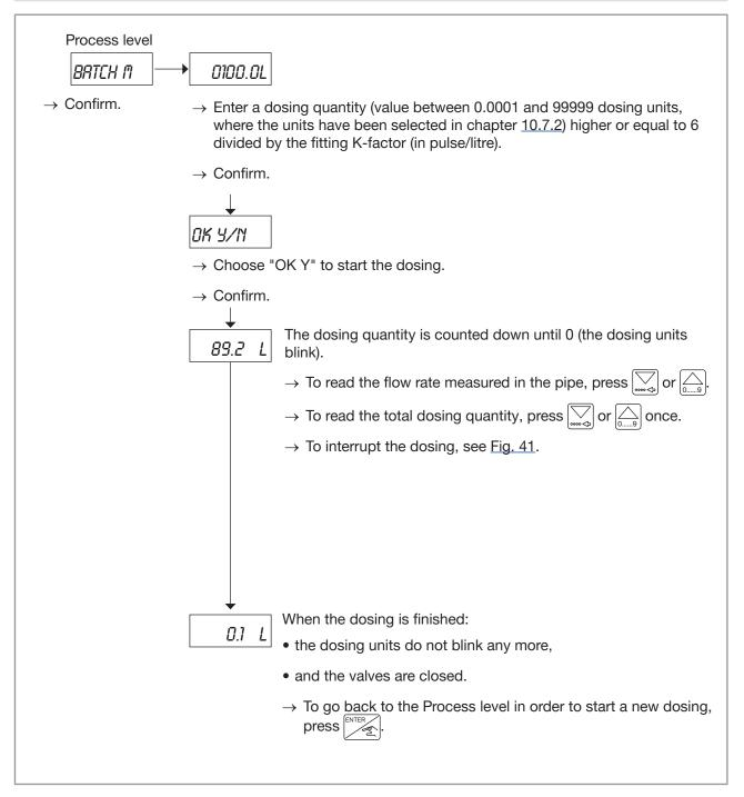
Fig. 40: Doing a manual dosing in dosing modes "LOC. MANU." or "MEM.+MANU."
