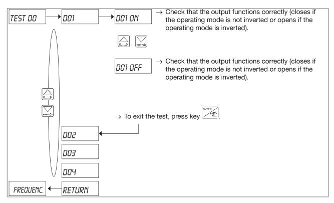
Fig. 95: Diagram of the "TEST DO" parameter of the Test menu
