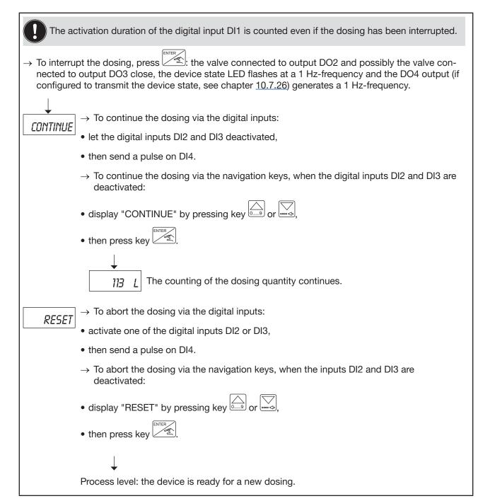
Fig. 51: Interrupting the dosing, in dosing mode "EXT. [T]"
