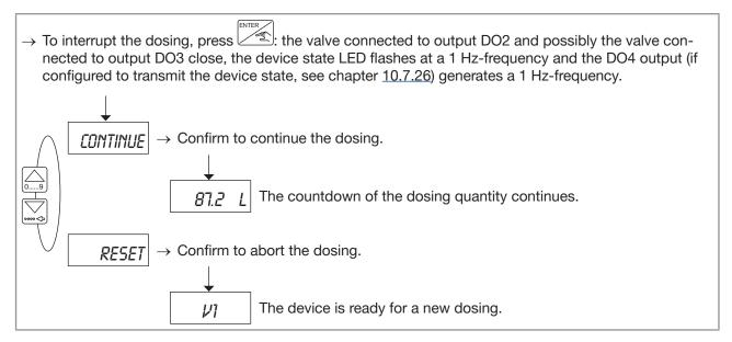
Fig. 43: Interrupting the dosing in dosing modes "LOC. MEM." or "MEM.+MANU."
