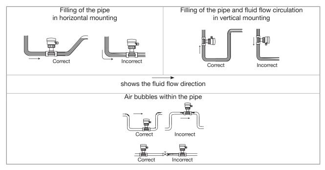
Fig. 11: Filling of the pipe, flow direction of the fluid, Vertical mounting Air bubbles within the pipe
