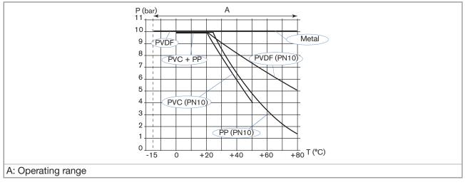
Fig. 8: Fluid temperature/fluid pressure dependency curves for the 8025 Batch in compact version, depending on the material the S020 fitting is made of
