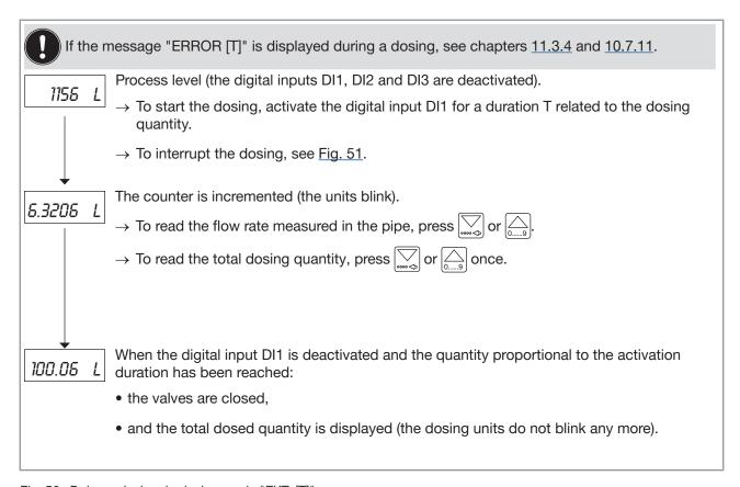
Fig. 50: Doing a dosing, in dosing mode "EXT. [T]"
