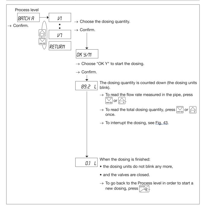
Fig. 42: Doing a dosing in dosing modes "LOC. MEM." or "MEM.+MANU."
