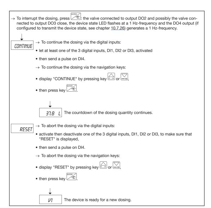
Fig. 49: Interrupting the dosing, in dosing mode "EXT.+LOC."
