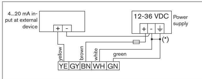
Fig. 15: Wiring the current output in sourcing mode on a version with cable gland
