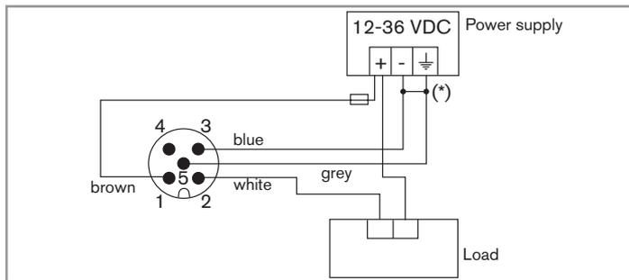
Fig. 8: NPN wiring (default) of the pulse output of a version with M12 fixed connector
