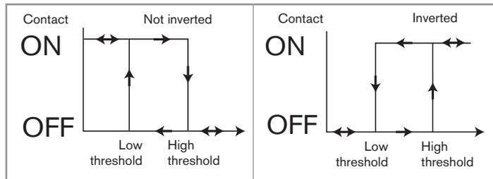
Fig. 16: NPN pulse output, hysteresis operating, non inverted and inverted
