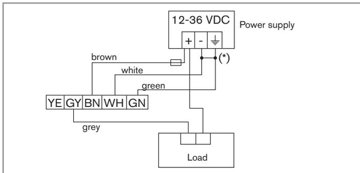
Fig. 12: NPN wiring (default) of the pulse output of a version with cable gland
