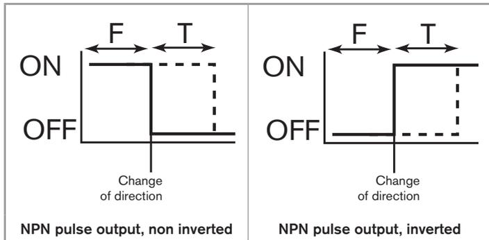
Fig. 20: Detection of the change in fluid circulation direction; NPN pulse output, not inverted and inverted
