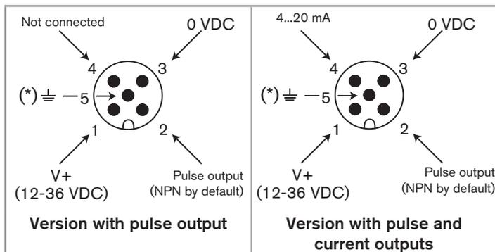
Fig. 7: Pin assignment of the M12 male fixed connector
