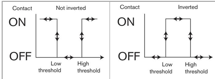
*Fig. 18: NPN pulse output, window operating, non inverted and inverted*
