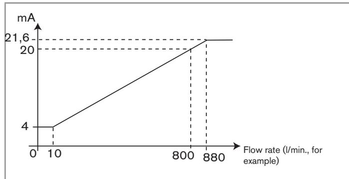
Fig. 24: Curve for the current proportional to the flow rate
