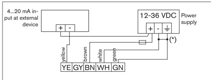
Fig. 14: Wiring the current output in sinking mode (by default) on a version with cable gland
