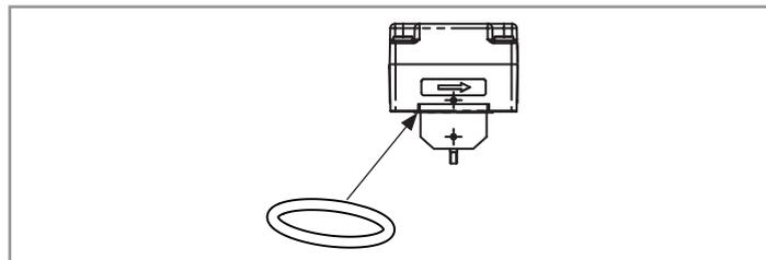
Fig. 27: Seal for metal fitting
