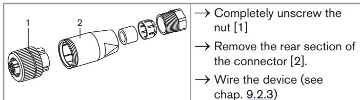
Fig. 6: M12 multi-pin connector (not supplied, ordering code 917116)
