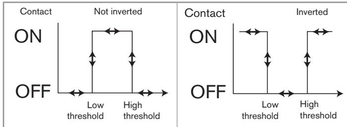
*Fig. 19: PNP pulse output, window operating, non inverted and inverted*
