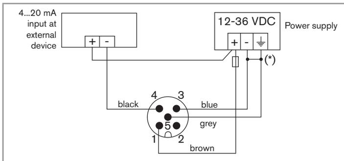
Fig. 10: Wiring the current output in sinking mode (by default) on a version with M12 fixed connector.
