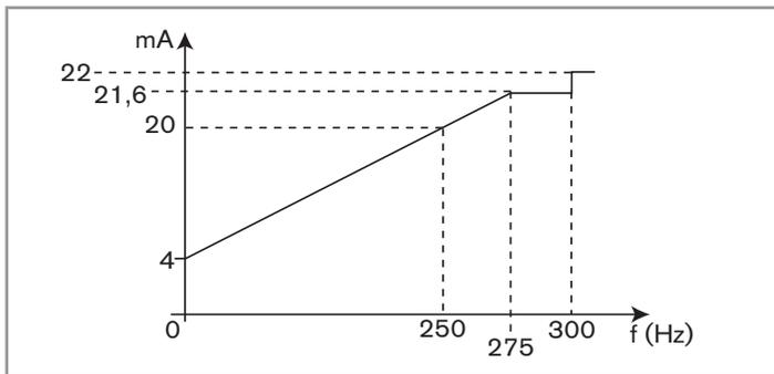
Fig. 23: Curve for the current proportional to the paddle-wheel rotation frequency
