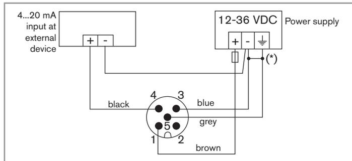
Fig. 11: Wiring the current output in sourcing mode on a version with M12 fixed connector
