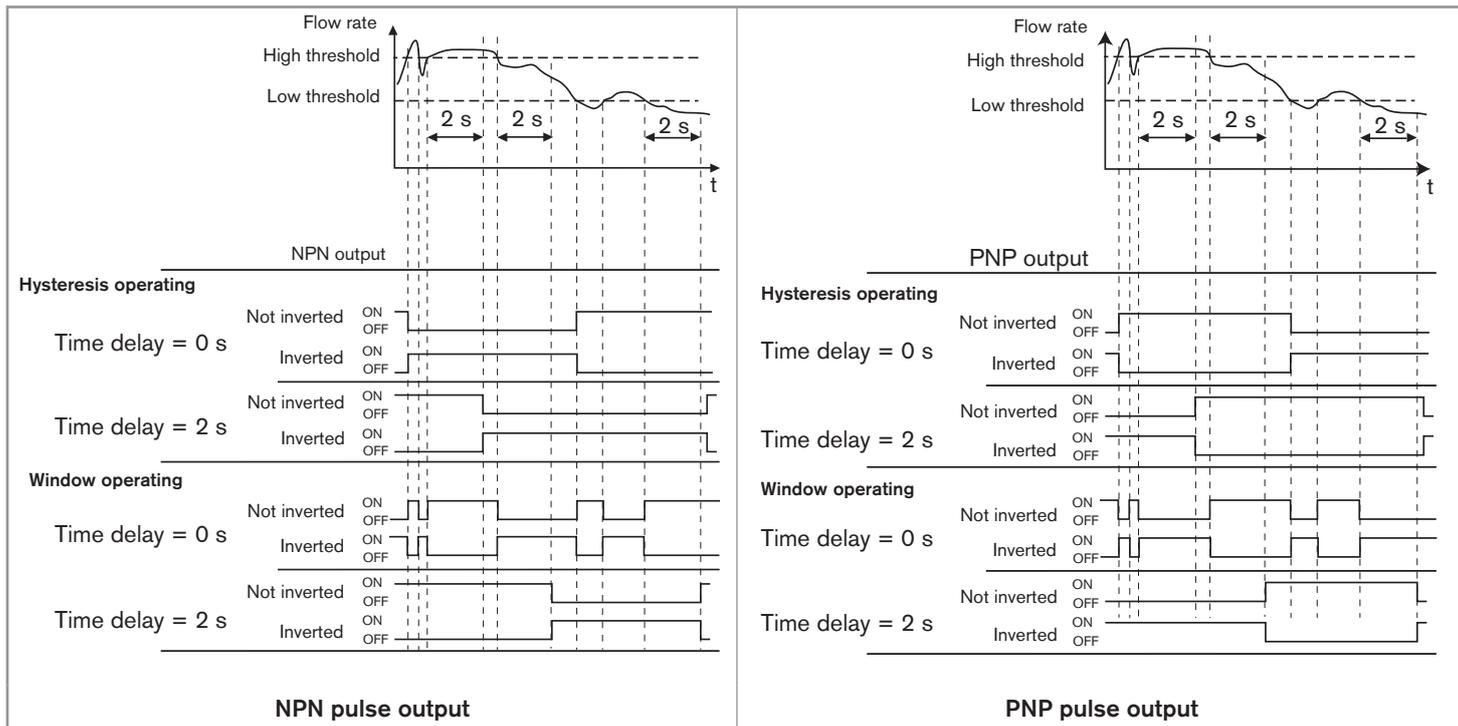
Fig. 22: Examples of behaviour of the 8012 depending on the flow rate in the pipe and the switching operating chosen for the pulse output
