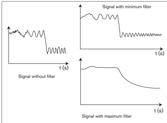
Fig. 25: Different filter levels for current fluctuations
