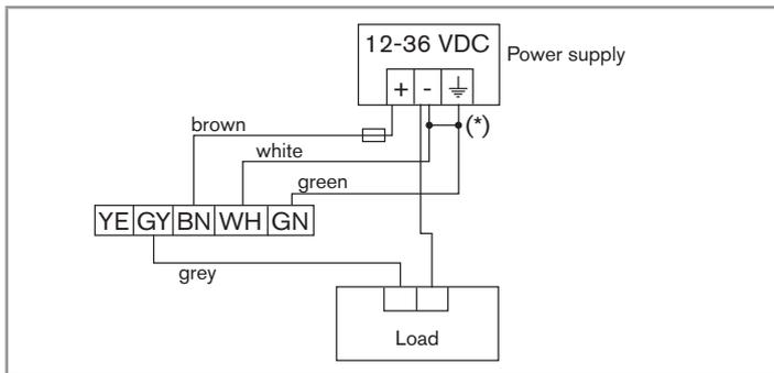
Fig. 13: PNP wiring of the pulse output of a version with cable gland
