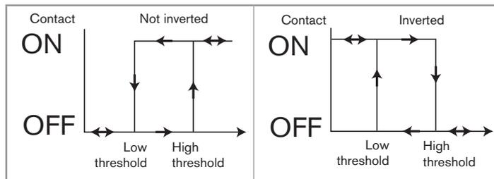
Fig. 17: PNP pulse output, hysteresis operating, non inverted and inverted
