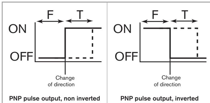
Fig. 21: Detection of the change in fluid circulation direction; PNP pulse output, not inverted and inverted
