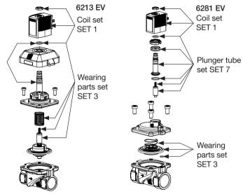
The composition of the spare part sets may differ from the diagram depending on the model of valves.
