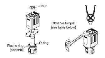
The rotational position of the coil on the valve body is arbitrary.
