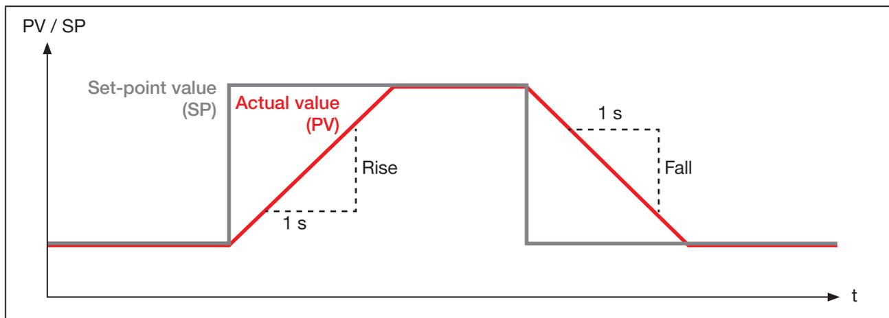
Figure 12: SP.SLOPE, effect of limit when there is a jump in the set-point value
