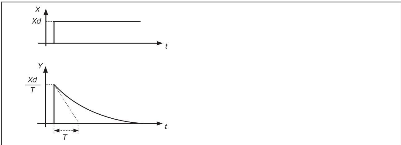
Figure 19: Characteristic of superposition of P, I and DT components
