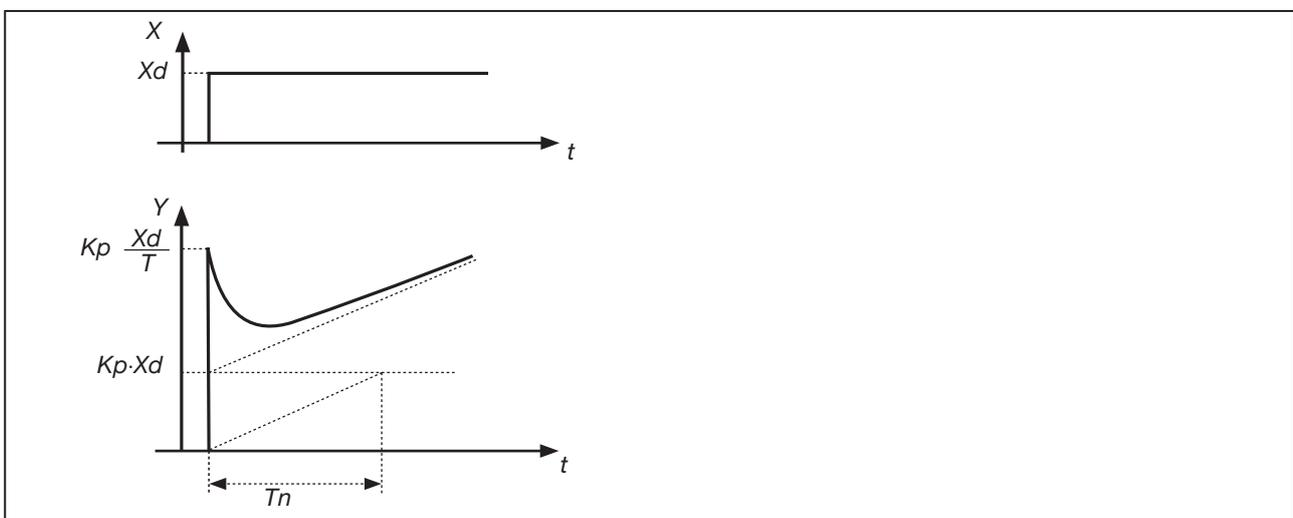
Figure 20: Characteristic of step response of the real PID controller
