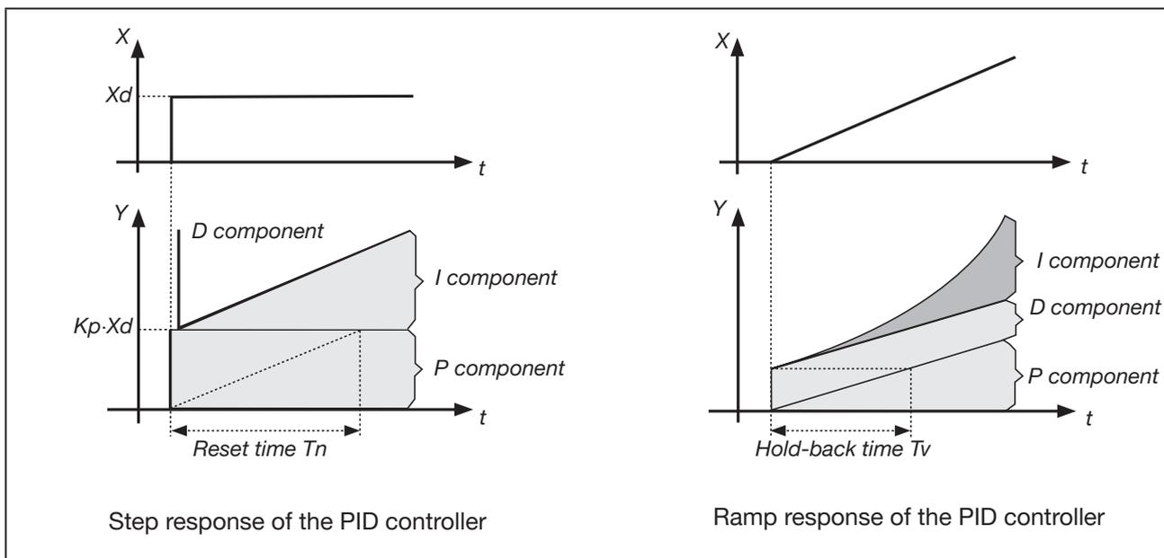
Figure 18: Characteristic of step response and ramp response of PID controller
