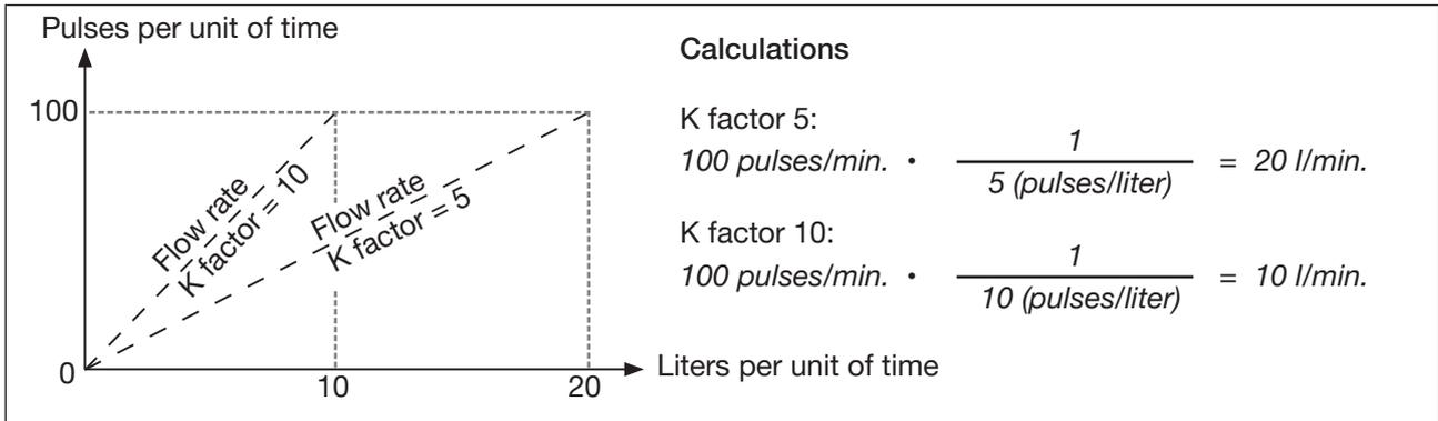
Figure 10: Example: K factor for sensor calibration for frequency signal type
