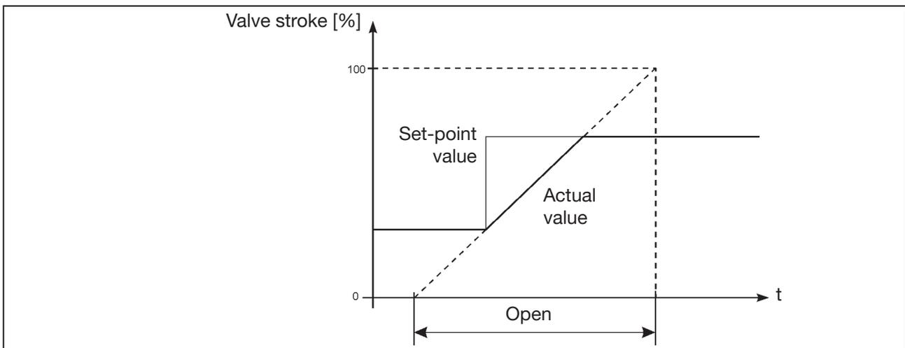
Figure 8: Diagram, limited opening speed
