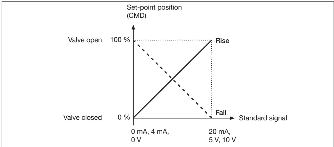
Figure 5: Diagram of effective direction
