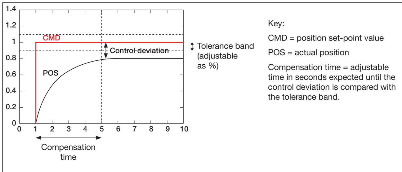
Figure 9: POS.MONITOR; schematic representation of position monitor
