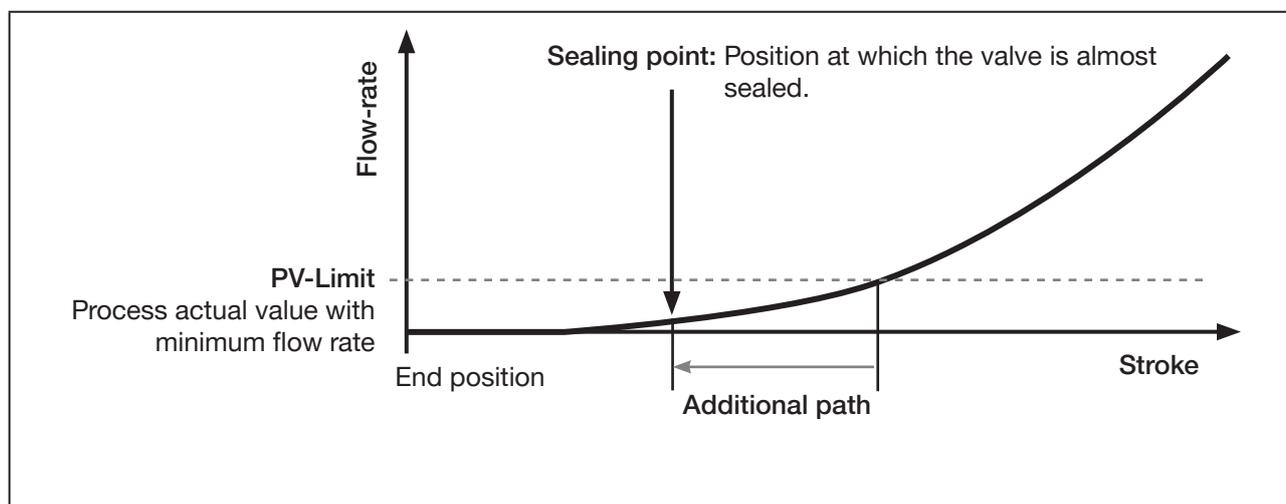
Table 24: Parameters for sealing function
