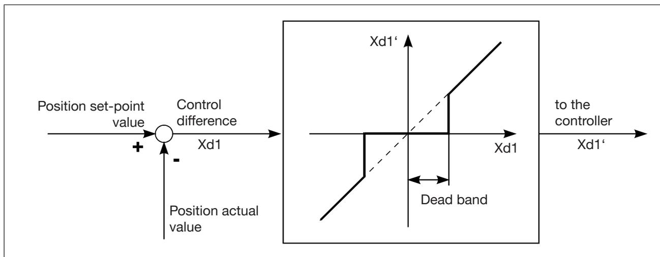
Figure 1: Diagram, insensitivity range
