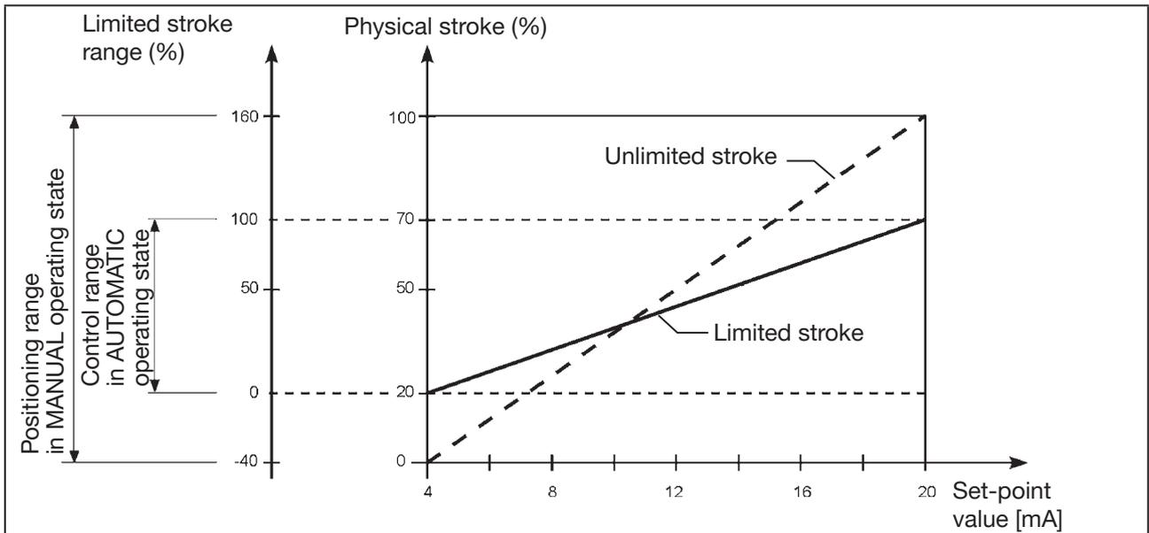
Figure 7: Diagram, mechanical stroke limit
