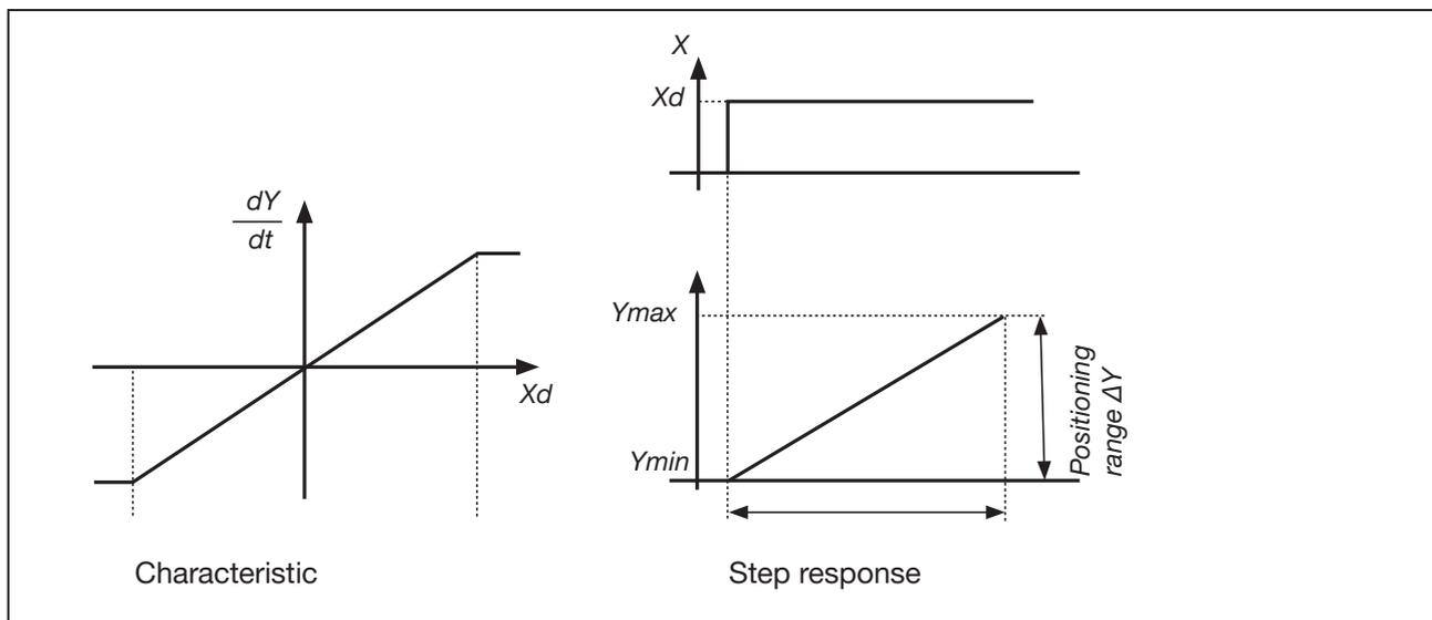
Figure 16: Characteristic and step response I component PID controller
