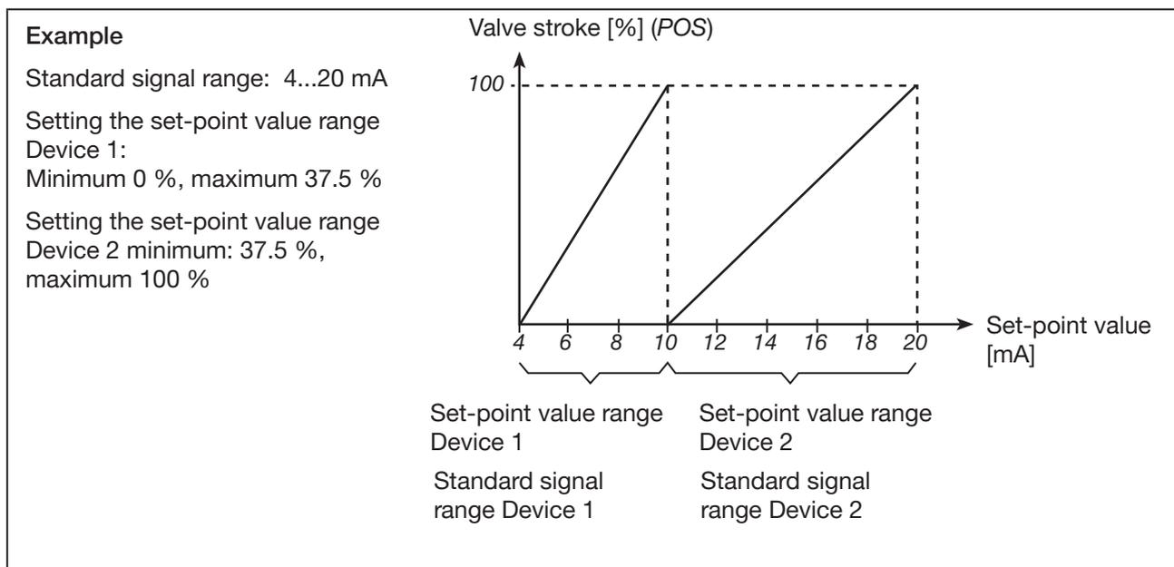
Figure 6: Diagram, signal split range
