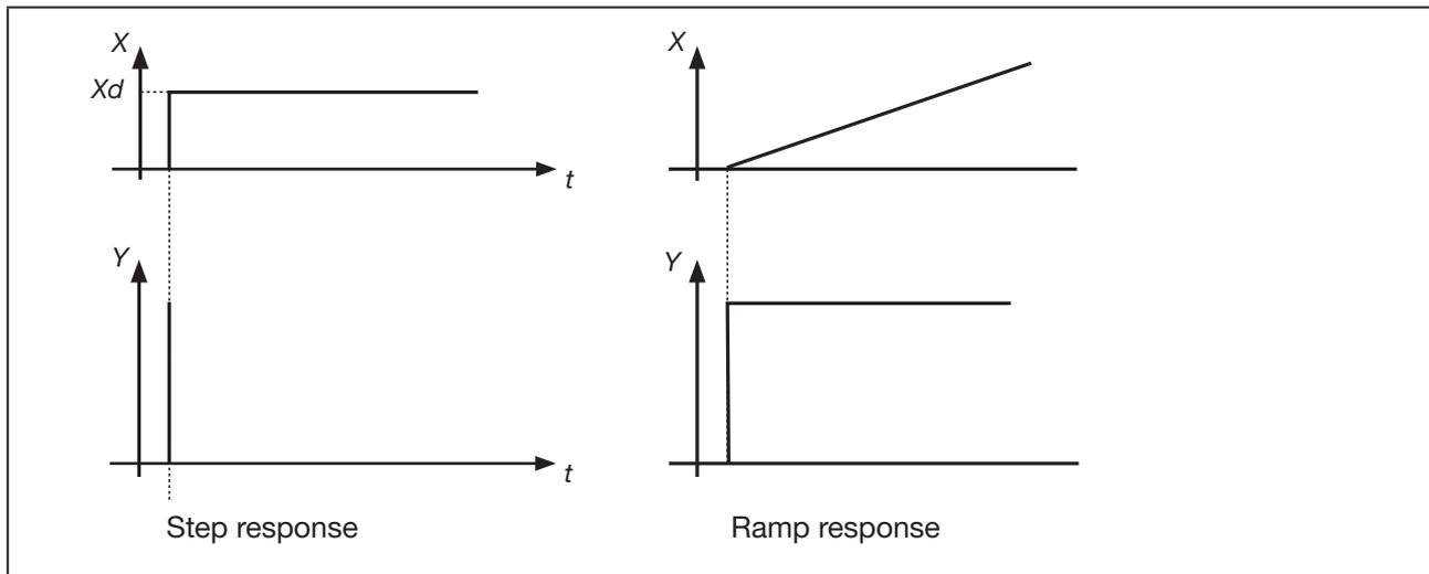
Figure 17: Characteristic and step response D component PID controller
