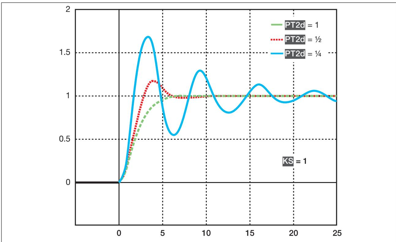
Figure 14: Example of different attenuations for a modeled process controlled system  $PT_2$
