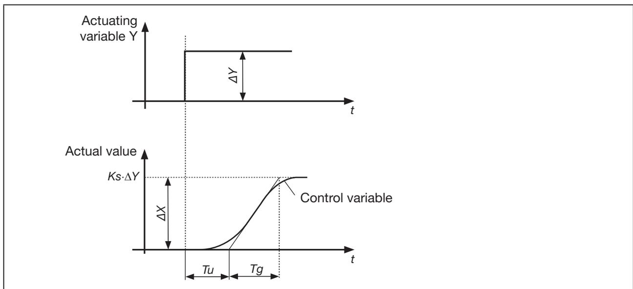
Figure 22: Progress of the control variable, actuating variable jump
