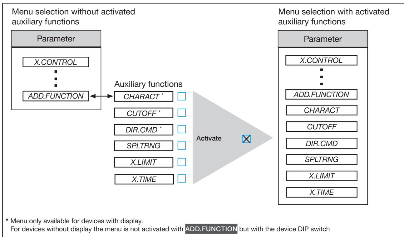
Figure 2: Activating the auxiliary functions
