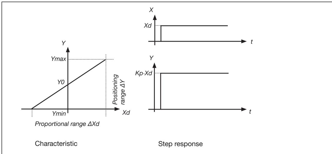
Figure 15: Characteristic and step response P component PID controller
