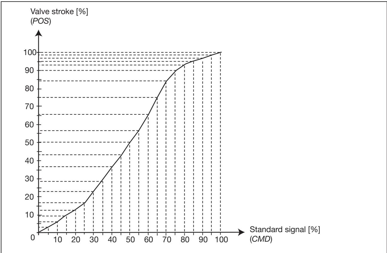
Figure 4: Example of a programmed correction characteristic
