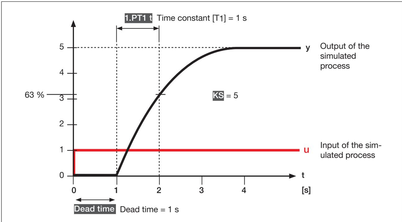
Figure 13: Example of a modeled process controlled system  $PT_1 - T_1$
