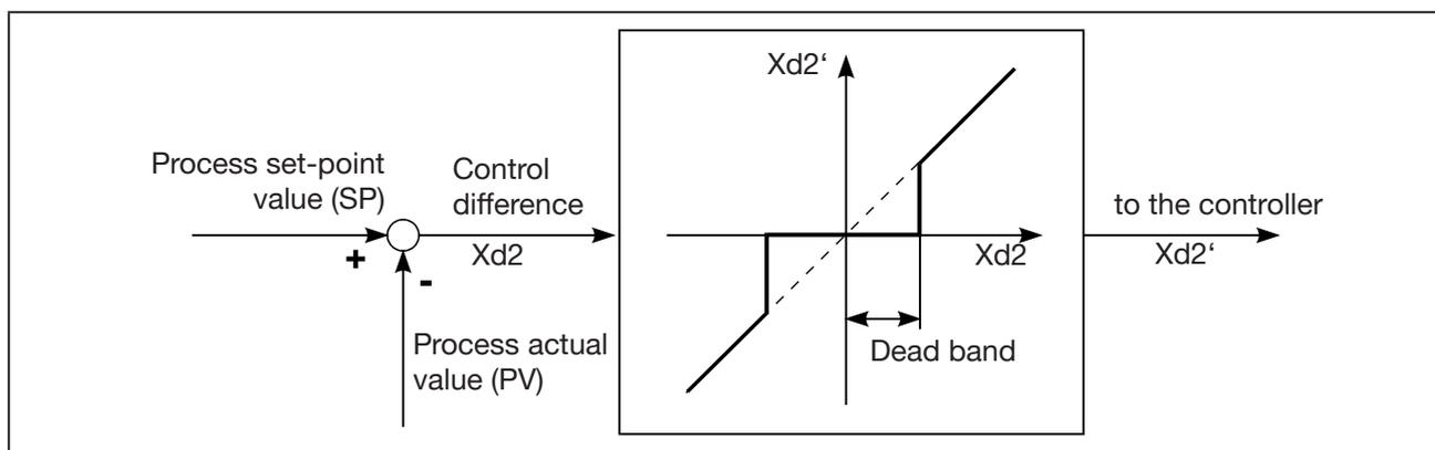
Figure 11: Diagram DBND; insensitivity range for process control
