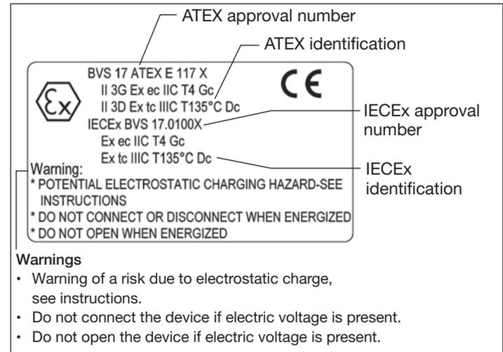
Fig. 4: Description: Adhesive label for the Ex area
