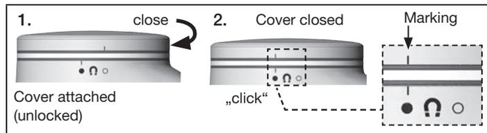
Fig. 3: Closing the dummy cover or display module
