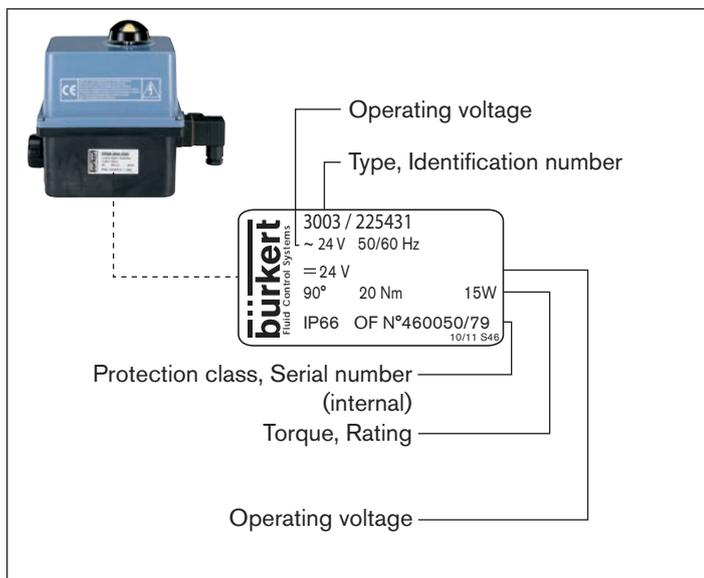
Fig. 1: Location and description of the type label
