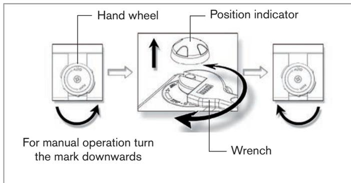
Fig. 12: Switching the rotary actuator from automatic to manual operation
