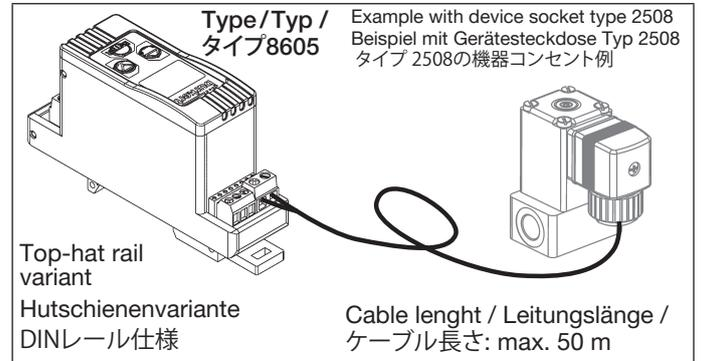
For plug designs with coil size 32 mm and 49 mm
