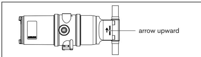
Fig. 4: Installation position for self-draining
