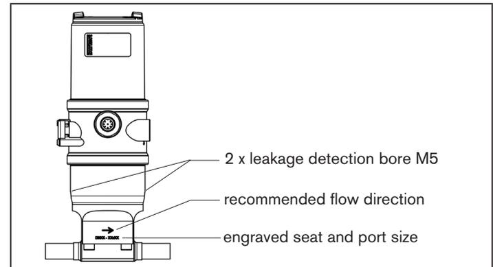
Fig. 3: Leakage detection bores and recommended flow direction
