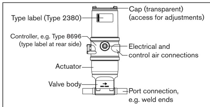
Fig. 1: General structure of Type 2380
