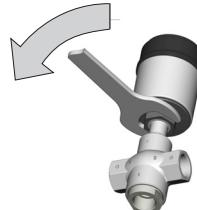
Fig. 3: Rotating the actuator
