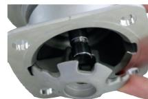
→ Clean pressure piece and lubricate spindle with suitable grease.
