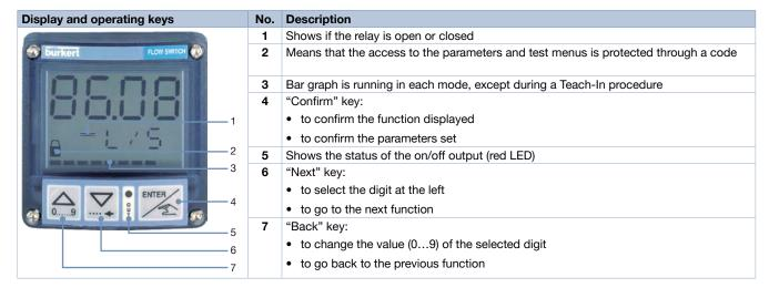
The device can be calibrated by means of the K-factor (conversion coefficient), or via the Teach-In function. User adjustments, such as engineering units, output, filter, bargraph are carried out on site.
